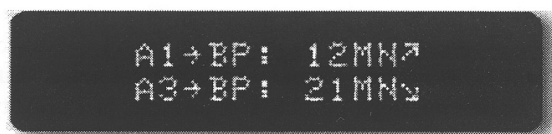
Fig. 5. A variable message sign (VMS) indicating travel times on alternate routes (Papageorgiou et al., 2003).
