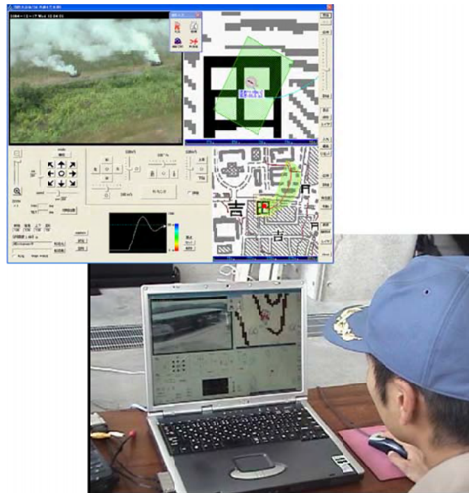
Fig. 7. Easy operation of the intelligent aerorobot with GUI on a note PC
