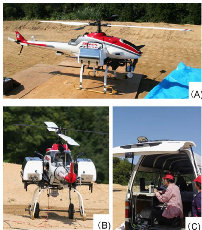
Fig. 6. Intelligent aerorobot by Kyoto University group (A) intelligent aerorobot's side view, (B) rear view, and (C) a van for robot transportation, equipped with control and monitoring devices.
