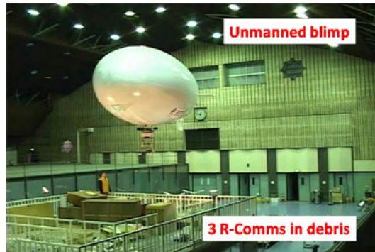
Figure 5. Communication test between blimp and R-Comm in indoor environment
