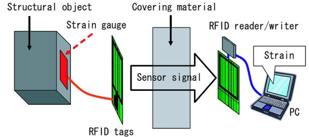
Fig. 1. Develop a structural health monitoring system using passive RFID tags
