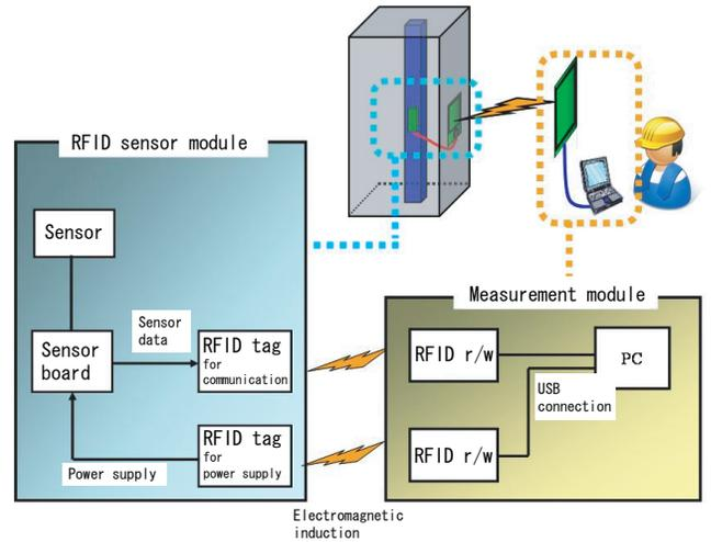
Fig. 2. Developed system architecture
