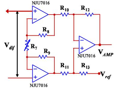
Fig. 4. Instrumentation amplifier circuit
