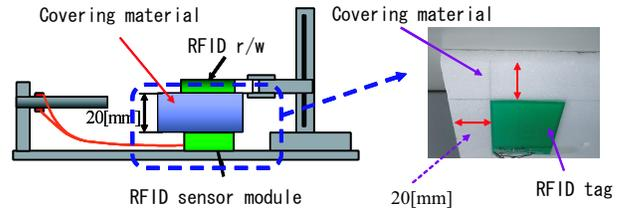
Fig. 11. Experimental equipment with covering materials
