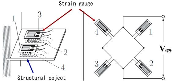
Fig. 9. Strain measurement using the four active gauge method
