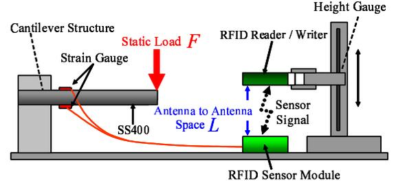
Fig. 7. Experimental equipment
