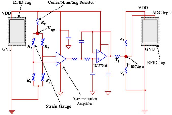
Fig. 3. Developed RFID sensor module circuit
