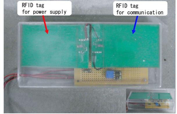
Fig. 5. Developed RFID sensor module
