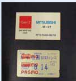
Upper: UHF-band RFID tag Lower: IC card (for comparison)
