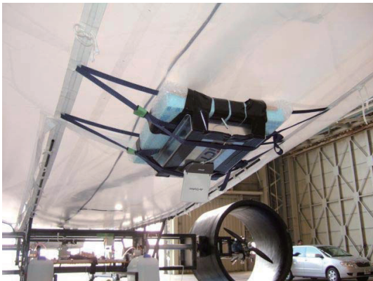
Figure 5 Collection device installed on the blimp
