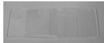
Figure 2 : A specimen from the construction material is set on the slide glass with the refractive index liquid and it is covered by cover glass (22mm X 22mm).
