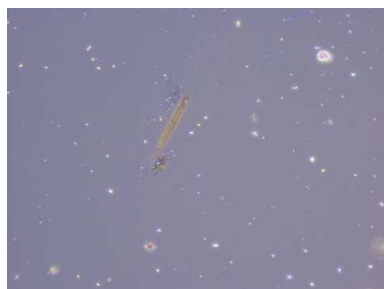
Fig. 1 Example of microscopic appearance of asbestos
