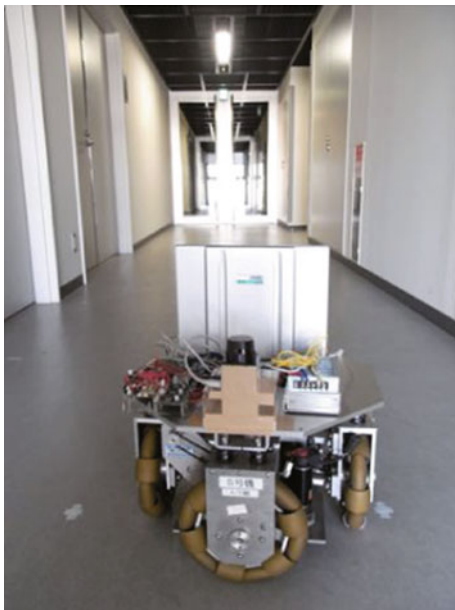
Fig. 6 Omni-directional mobile robot used in the experiments
