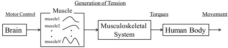
**Fig. 4** The figure indicates model of human body movement. Firstly, brain sends motor control signals into muscles to exert forces by flexion or extension. Next, each muscle generates torque to human joints and human body moves according to its dynamics.
