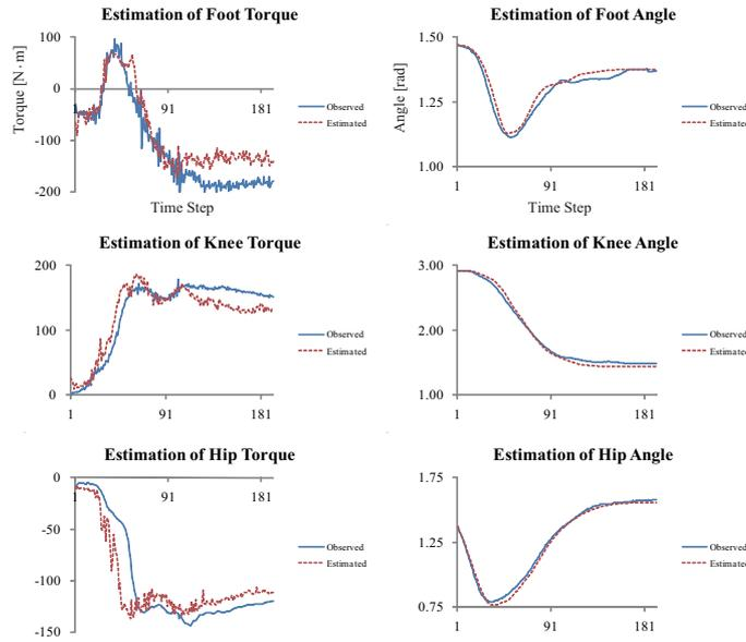
**Fig. 7** Example of estimation of three joint torques and joint angles from the same trial. Left three graphs are results of torque estimation and right three graphs are ones of angle estimation. Blue solid line is observed data and red dotted line is estimated data.
