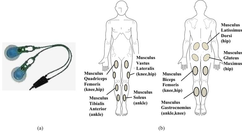
**Fig. 3** (a) Two sEMG monopolar electrode sensors were used to measure each muscle. (b) Sixteen muscles were measured (eight muscles for the each half body). Above figure illustrates positions of measured muscles and joints of muscle attachment.
