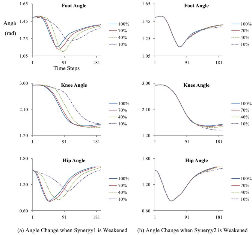
**Fig. 10** Graphs indicate how each joint angle change with weakened synergies. Left three graphs show values when synergy1 was weakened, and right ones show values when synergy2 was weakened. X-axis represents a time step (1/64 sec) and y-axis represents angle (rad).
