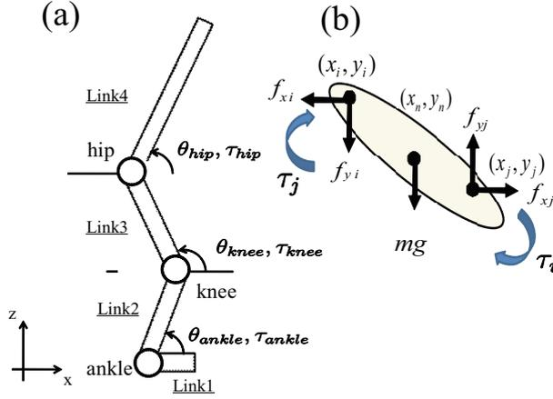
**Fig. 5** (a) The link model used in our research to express human body. Each link expresses feet (Link1), lower legs (Link2), upper legs (Link3), and upper body (Link4) and joints between links are ankle, knee, and hip. (b) indicates variables used in computation of torques.
