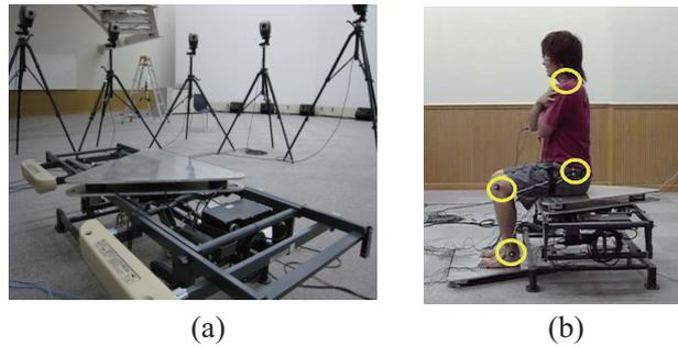
**Fig. 1** (a) A motion capture machine with eight cameras [HMK-200RT; MotionAnalysis] was used in our experiment to record body position. (b) Four points were recorded during the experiments: ankle, knee, hip, and shoulder.
