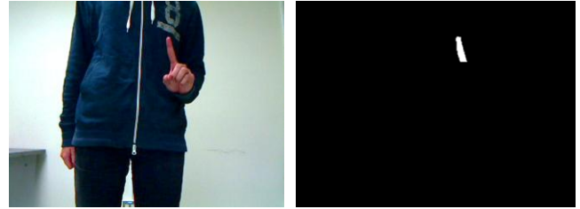
(a) Acquired image. (b) Finger region. Fig. 10 Appearance at a distance of 50cm.
