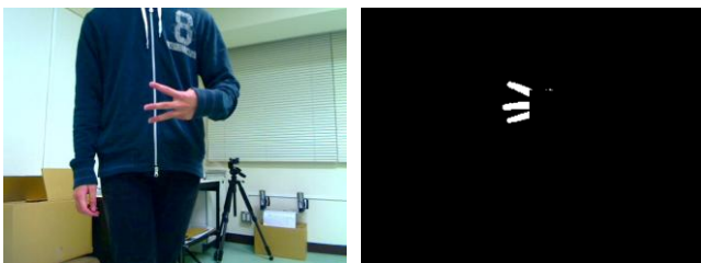
(a) Acquired image. (b) Finger region. Fig. 14 2nd movement directive: 180 degrees turn.
