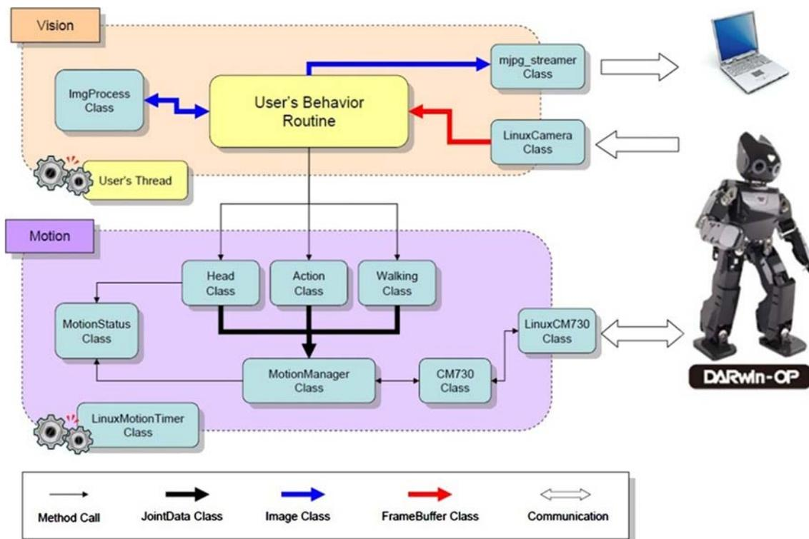
Figure 9. Software framework pipeline for DARwIn-OP.
