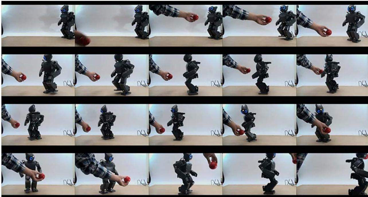
Figure 12. Movie captures of walking test of DARwIn-OP.
