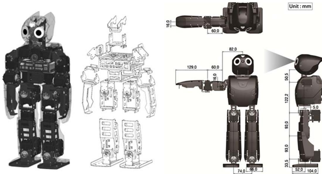
Figure 4. Mechanical design of DARwIn-OP.
