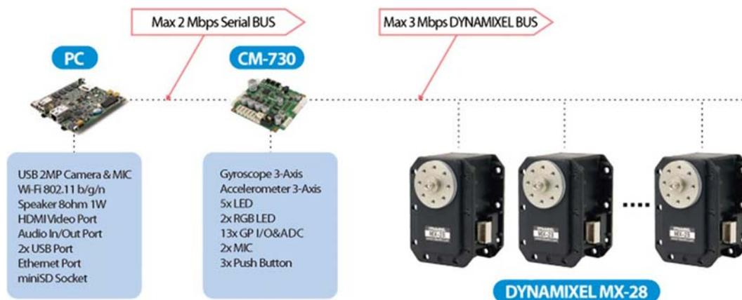
Figure 2. Modularized component of DARwIn-OP based on PC architecture.
