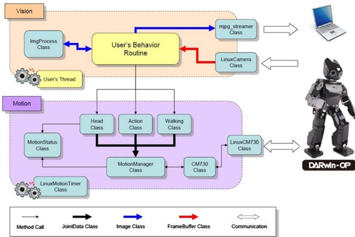
Figure 9. Software framework pipeline for DARwIn-OP.
