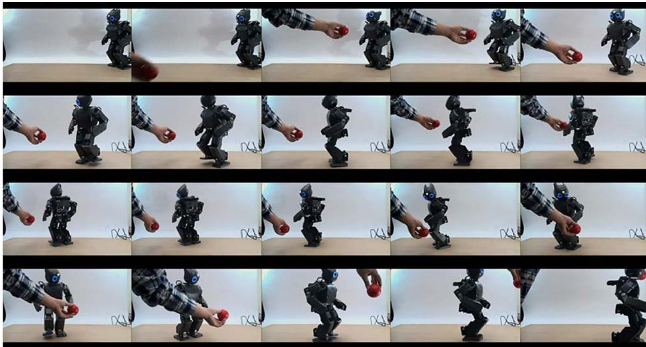
Figure 12. Movie captures of walking test of DARwIn-OP.
