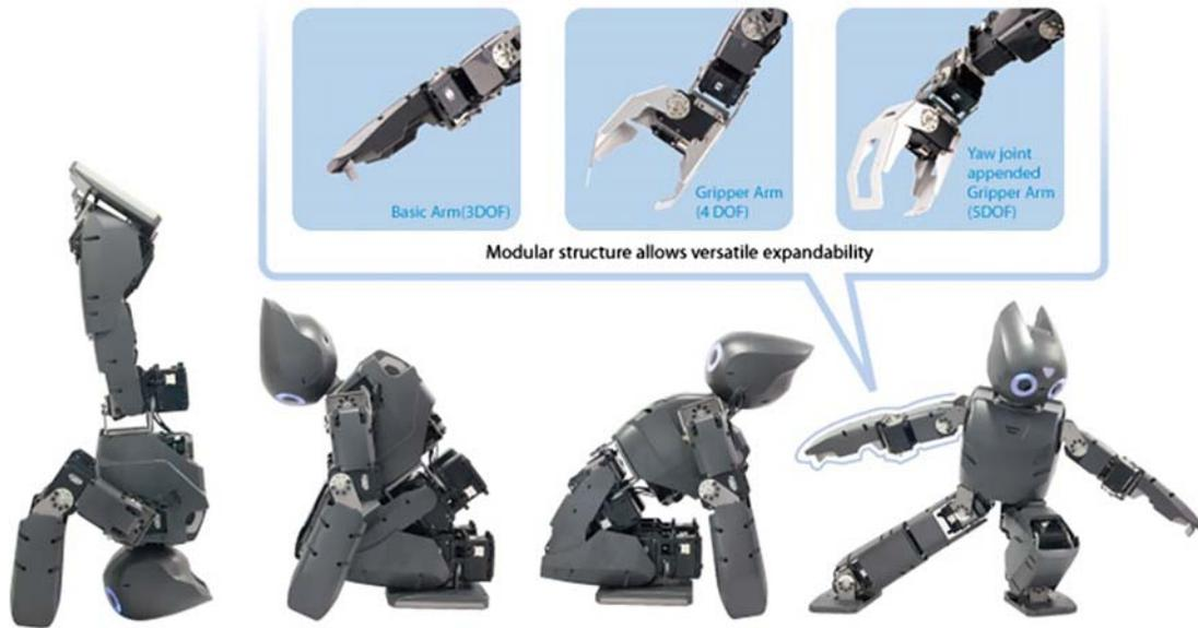
Figure 5. Different types of grippers for DARwIn-OP.
