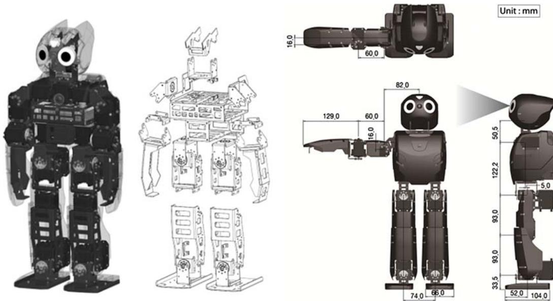
Figure 4. Mechanical design of DARwIn-OP.
