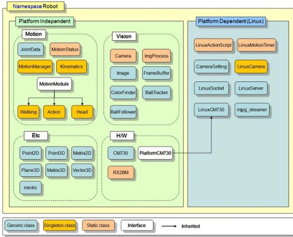
Figure 8. Software framework class diagram for DARwIn-OP.
