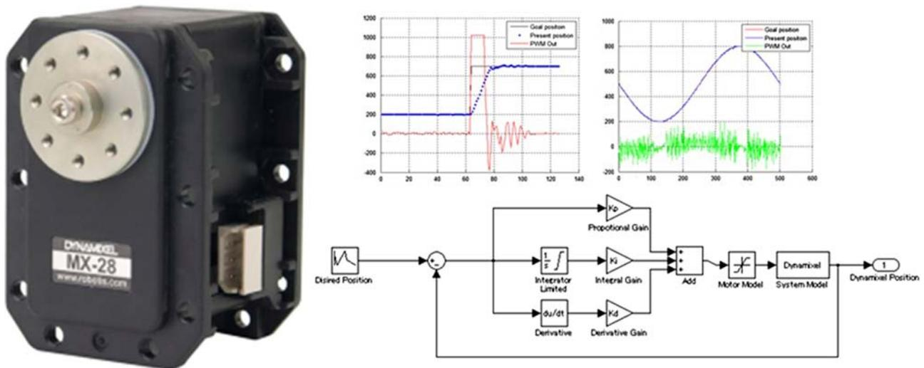
Figure 6. Developed MX-28 actuator for DARwIn-OP.
