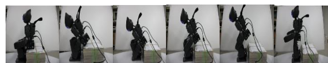
step1 step2 step3 step4 step5 step6 Fig. 1 Sit-to-Stand motion of the robot.
