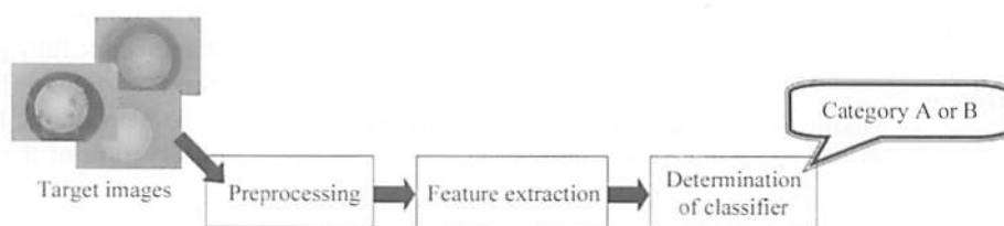
Figure 4 Processing flowchart of the method presented here. The method consists of preprocessing, feature extraction and classification.
