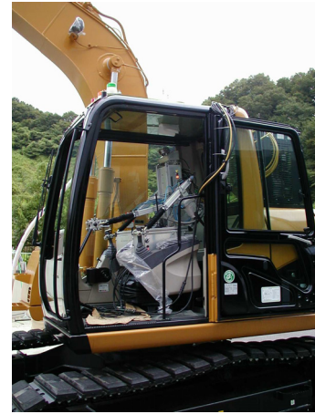
Fig. 3. Remote-controlled Robo Q robot.
