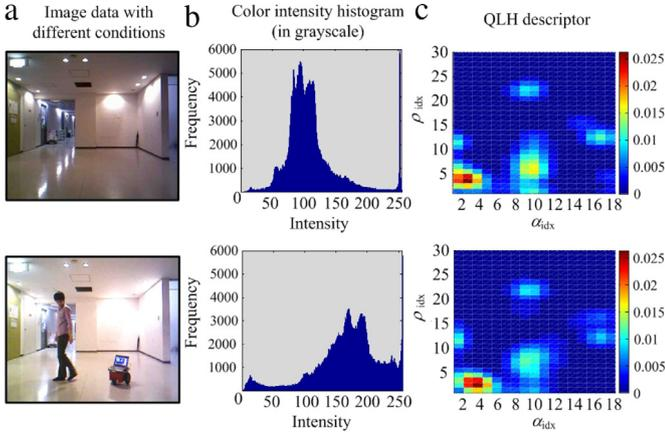
**Fig. 14.** Examples of image matching criteria: (a) original images, (b) color intensity histograms, and (c) QLH descriptors.
