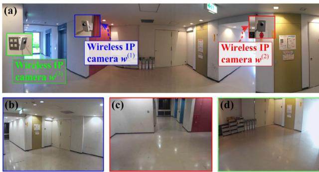
**Fig. 22.** Experimental environment with wireless IP camera network: (a) real environment, (b) real image data from wireless IP camera  $\mathbf{w}^{(1)}$ , (c) real image data from wireless IP camera  $\mathbf{w}^{(2)}$ , and (d) real image data from wireless IP camera  $\mathbf{w}^{(3)}$ .
