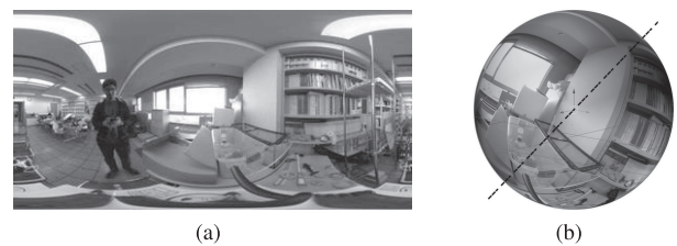
Fig. 1 An example of a complete spherical image in (a) equirectangular projection (b) spherical projection. They can be rotated in any direction without information loss.
