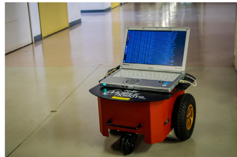
Fig. 5. Hardware configuration for data acquisition: CZ-SZ5 laptop and a Pioneer 3 DX.
