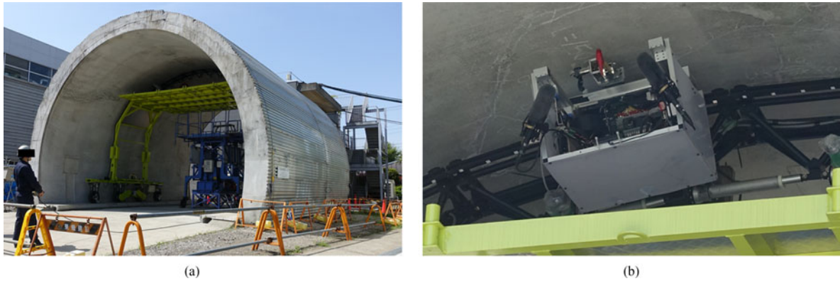
Fig. 10. Field conditions experimental setting. (a) Mock tunnel: located outdoors and in real scale, this tunnel exhibits naturally occurred defects and closely matches real-life field conditions. (b) Hammering module mounted on Variable Guide Frame: this system allows automatic hammering and data collection anywhere inside a tunnel [17]–[19].
