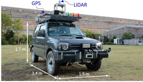
Fig. 10. Suzuki Jimny customized for fully autonomous driving on rough terrain, which is assumed as off-road UGV in experiments.
