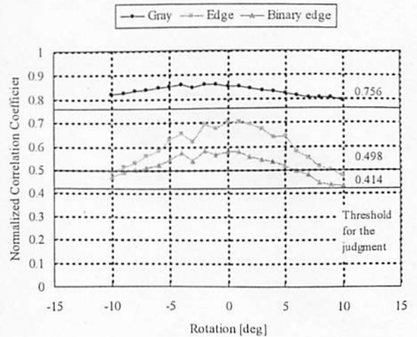
図 15 未知画像の回転角度と正規化相関係数の関係 Fig. 15. Relationship between rotation of unknown image and normal correlation coefficient.
