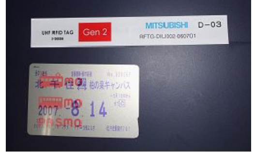
Fig.4 RF-tag for attachment to metal with a smart card for comparison
