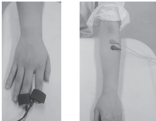
Fig. 2 Experimental condition for the EMG and SCR measurement
