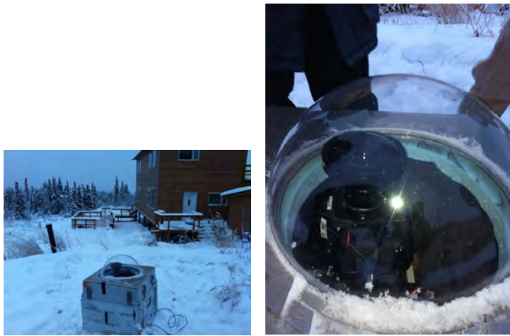
(a) Outward appearance of fisheye camera system (b) Inside of fisheye camera system
