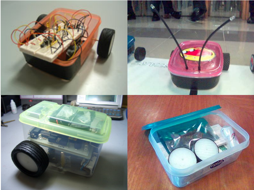
Figure 14: Clockwise from upper left – First prototype of RoboBOX, Start/basic kit, RoboBOX components in unassembled form, GoGoBOX
