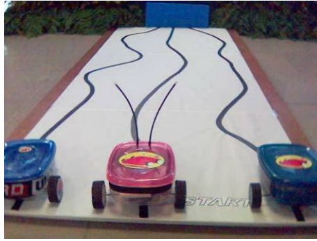
Figure 3: RoboBOX as line follower robot
