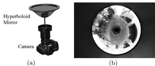
**Fig. 1** Omnidirectional camera. (a) Camera with a hyperboloid mirror. (b) Acquired image.
