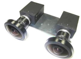
Fig. 9 Fish-eye stereo camera
