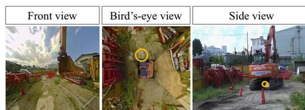
Fig. 20 Example images in controlling stop position experiment. Yellow circles indicate stop marks. Bird's-eye view can show a backhoe and a stop mark relatively.
