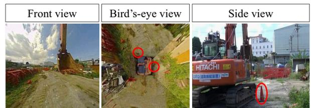
Fig. 18 Example images in moving narrow path experiment. Red circles indicate obstacles. Bird's-eye view can show both of obstacles.
