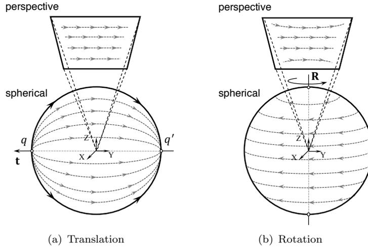
Figure 2. Optical flow on spherical and planar projections. (a) Spherical and perspective optical flow with the pure translational movement of  $\mathbf{t}$  (from  $q$  to  $q'$ ) of a spherical camera, and (b) the pure rotational movement of  $\mathbf{R}$  to the counterclockwise direction.
