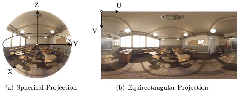
Figure 1. Spherical cameras can capture images as (a) spherical and (b) planar equirectangular projections owing to their  $360^\circ$  field-of-view.
