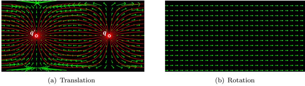
Figure 3. Optical flow computation results. The optical flow in the equirectangular projection with (a) the pure translation from  $q$  to  $q'$ , and (b) the pure yawing rotation. The optical flow with the pure translation are seen that they are aligned along the red curved lines, indicating the epipolar curves.
