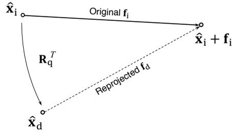
Figure 4. The initial optical flow vectors  $\mathbf{f}_i$  are derotated using the rotation matrix of quaternion  $\mathbf{R}_q^T$ , and then the reprojected optical flow vectors  $\mathbf{f}_d$  are obtained.
