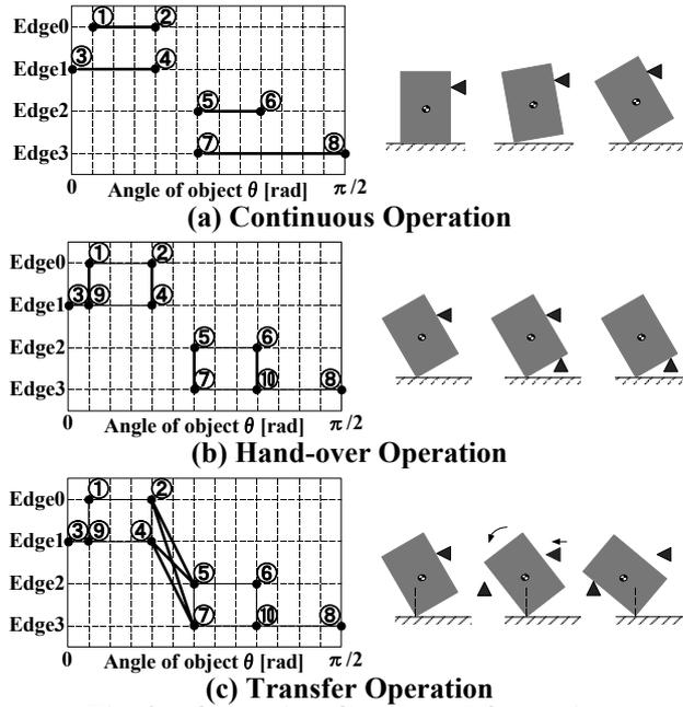
Fig. 8 Operation Graph and Operation
