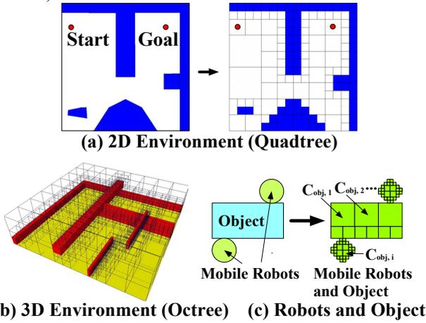
Fig. 10 Representation by Cell Decomposition
