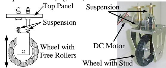
Figure 2. Developed wheel unit
