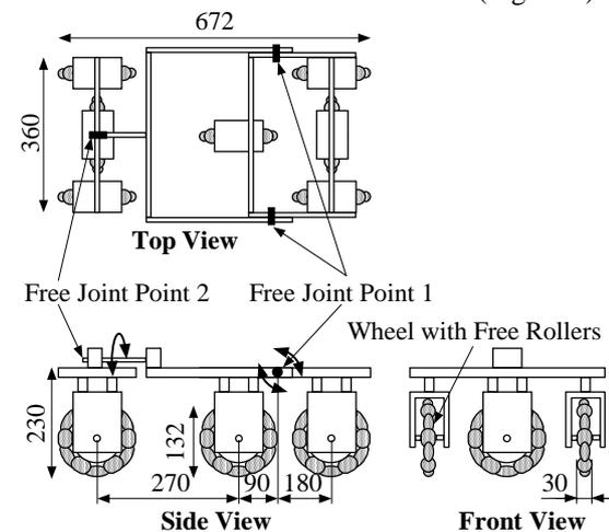
Figure 3. Mobile robot with seven universal wheels
