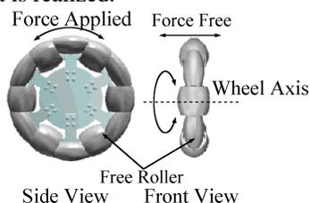
Figure 1. Universal wheel with free rollers
