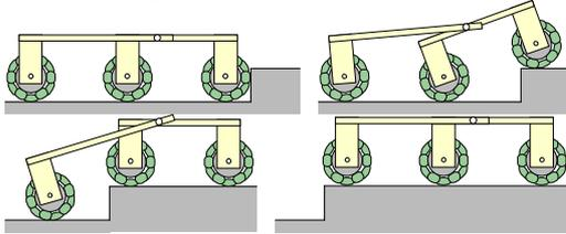
Figure 5. Process of climbing up a large step
