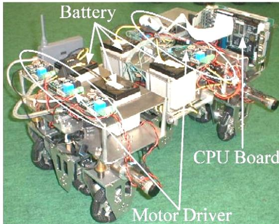
Figure 7. A prototype mobile robot
