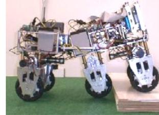
Figure 8. Experimental view of step climbing
