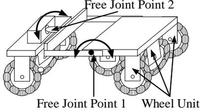
Figure 4. Passive suspension system of a robot
