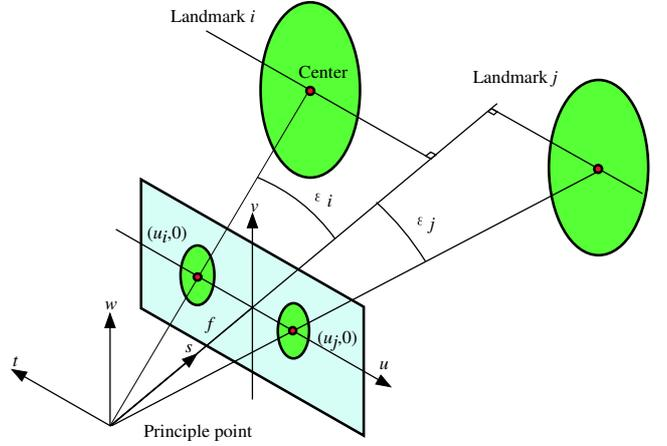
Fig. 10: Image of landmarks in the case of three-landmark observation. There is one image that projects more than two landmark and one image that projects more than one image.
