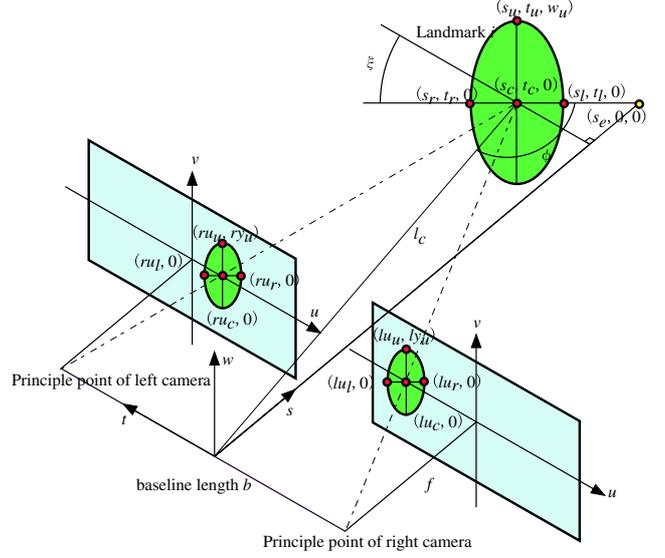
Fig. 6: Image of landmark in the case of stereo observation.
