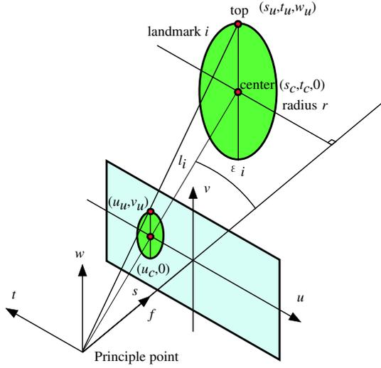
Fig. 8: Image of landmark in the case of two-landmark observation. There are two images that project one landmark.
