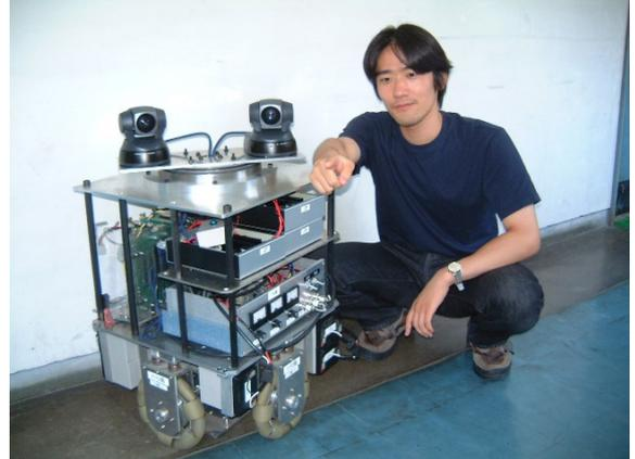
Fig. 2: Mobile robot system. An omni-directional mobile robot mechanism [11] is adopted as the robot base and two pan-tilt-zoom cameras that can change their direction independently are set on the top of the robot.
