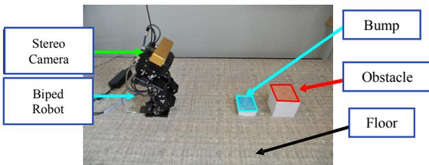
Fig. 2 Biped robot equipped with a stereo camera system.
