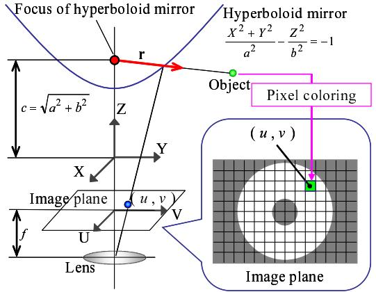
Figure 6. Calculation of ray vector and pixel coloring. A ray vector  $\mathbf{r}$  is defined as a unit vector which starts from the focus of the hyperboloid mirror. The point at which the ray vector intersects with the 3D model is calculated. The pixel color at the image coordinates  $[u, v]^T$  is determined as the same color of the cross-point.
