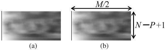
Figure 9. Autocorrelation images generated from the same location. (a) An autocorrelation image generated from a location. (b) An autocorrelation image generated from the same location with camera rotation by 90 degrees.
