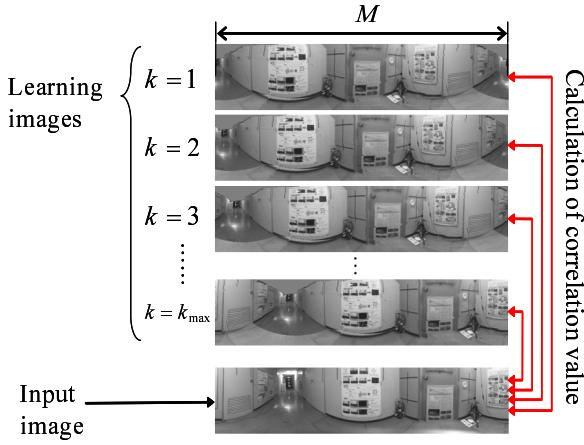
Figure 10. Pose estimation method. A learning panoramic image is shifted little by little. The correlation values between the input panoramic image and the shifted images are calculated.
