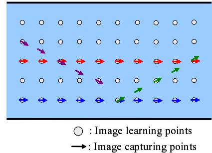
Figure 14. Input images capturing points. Input images are captured at the location of arrows. 10 input images are captured along the same path where the robot moved beforehand (red arrows). 20 input images are captured along the other path (purple, green and blue arrows). White points are image learning points.
