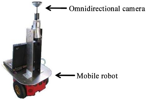
Figure 3. Mobile robot equipped with an omnidirectional camera.
