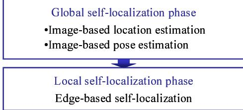
Figure 5. Navigation process. The self-localization is composed of two phases: autocorrelation image matching (global self-localization) and 3D-2D edge matching (local self-localization).
