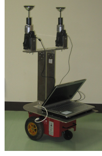
Figure 12. The mobile robot equipped with two omnidirectional cameras.
