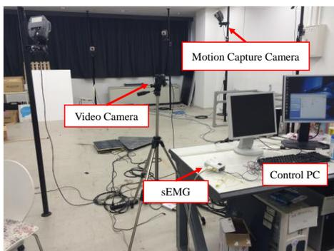
Fig. 3 Measurement devices
