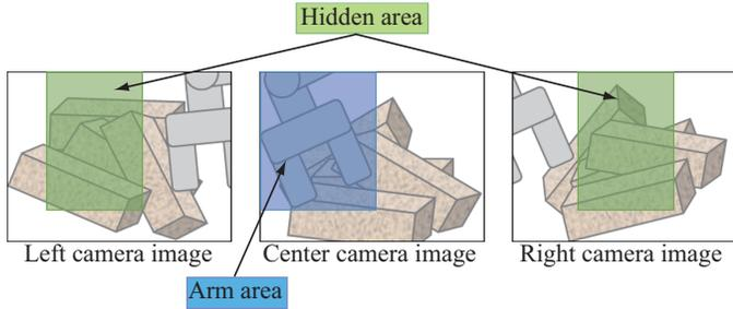
Fig. 3. Definition of each area in camera images. An area of the robot arm in the center camera is defined as an arm area, and areas occluded by the robot arm area in the other camera images are defined as hidden areas.
