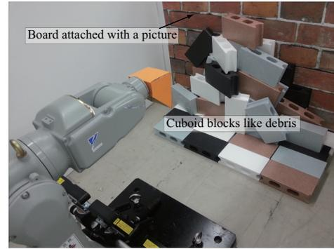
Fig. 9. Background objects. Two types of objects are used in the experimental environment. The first type was the board attached with a picture. The second type is comprised of cuboid blocks similar to debris scattered in front of the board.
