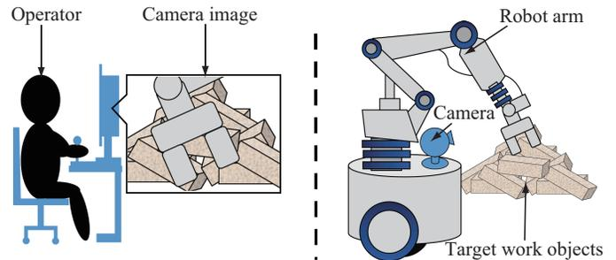
Fig. 1. Remote control system of a robot. Operators control robots remotely with the aid of a mounted camera. However, some target work objects are occluded by the robot arm in the camera image. Therefore, the operating efficiency decreases significantly.
