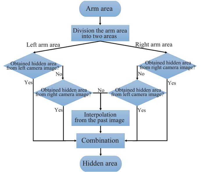
Fig. 5. Flow chart of procedures for obtaining the hidden area occluded by arm area in the center camera
