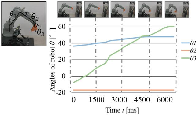
Fig. 8. This graph shows the orbit of the robot. Joint angles of the robot are defined in this image, and the robot copied debris the removal motion.
