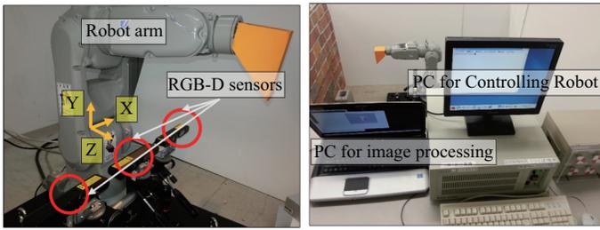
(a) Positions about RGB-D sensors and the robot arm (b) General view of this experimentation
