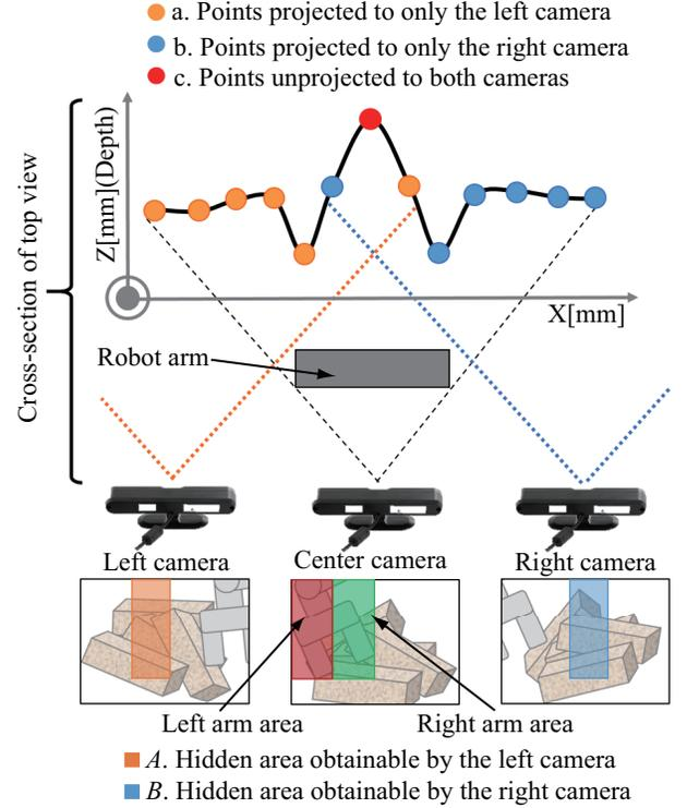
Fig. 4. Top view of experimental conditions. The points in this image indicate surficial shapes of the target work object occluded by the robot arm in the center camera and, they are classified into the specified three types.
