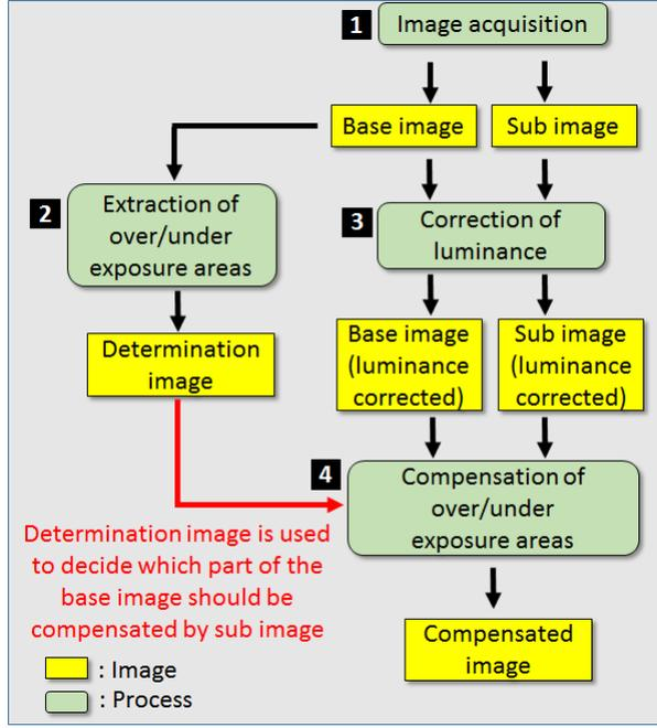
Fig. 2. The schematic view of our proposed method for compensation of over/under exposure using two images obtained in multiple lighting system.
