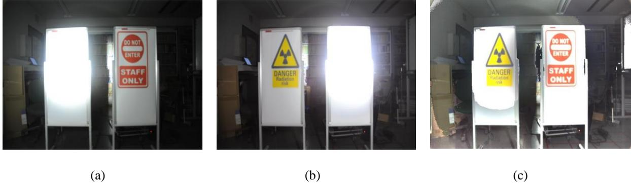
Fig. 8. Experiment result : (a)The base image  $I_0^{\text{base}}$  which is used in the experiment, (b)The sub image  $I_0^{\text{sub}}$  which is used in the experiment, (c)The compensated image  $I_c$  which is obtained by the proposed method.
