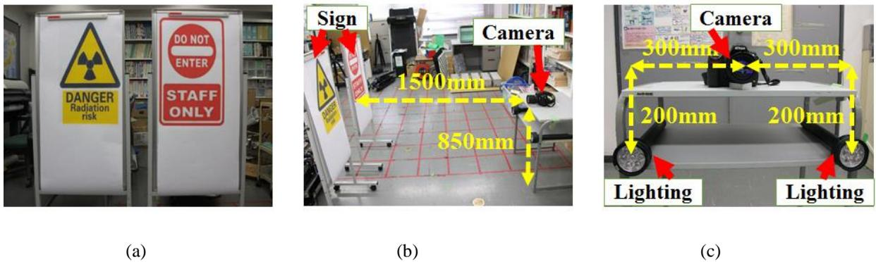
Fig. 7. Experiment environment : (a)Two signs which were used in the experiment, (b)The distance between the signs and the camera, (c)The distance between the camera and the lightings.
