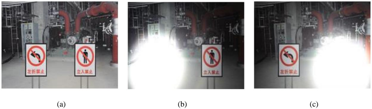
Fig. 3. Images obtained in image acquisition step : (a)The background image, (b)The base image  $I_0^{\text{base}}$  which can be obtained by turning on the left lighting, (c)The sub image  $I_0^{\text{sub}}$  which can be obtained by turning on the right lighting.
