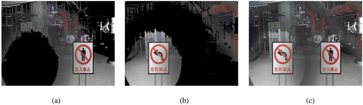
Fig. 6. Images obtained in compensation of over and under exposure areas step : (a)The output areas from the base image, (b)The output areas from the sub image, (c)The compensated image  $I_f$ .
