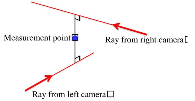
Fig. 5: Measurement point
