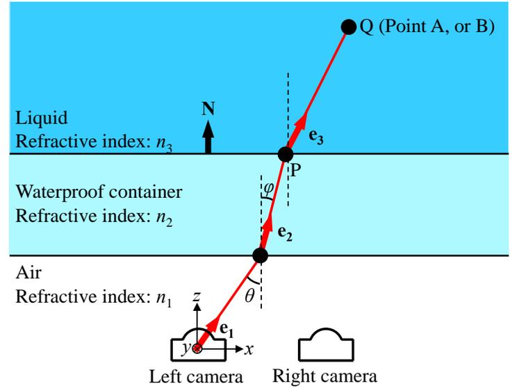
Fig. 4: Refraction of light
