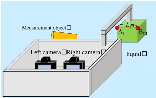
Fig. 2: Measurement system
