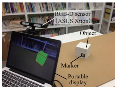
Fig. 5. Experimental setup. An RGB-D sensor for obtaining RGB images and 3D point clouds. An Object on which a marker has been placed is displayed on a portable display with overlaid virtual objects.
