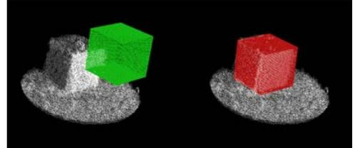
Fig. 4. Point cloud alignment using ICP. Before the alignment, the points extracted from the object's shape model (green points) do not match the object cloud (left image). By applying ICP to these points, the aligned points (red points) are adjusted to the points corresponding to the physical object (right image).
