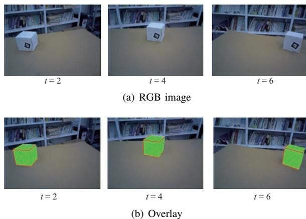
Fig. 7. Case 2: the marker is installed at the bottom right on the front surface for rotation around the normal line of the cube surface
