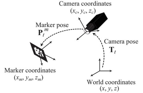
Fig. 2. Camera pose tracking. In this paper, camera and marker pose are defined as the transformation matrix that expresses the transformation between the two coordinates. Camera pose is estimated based on the assumption that markers on objects never move.
