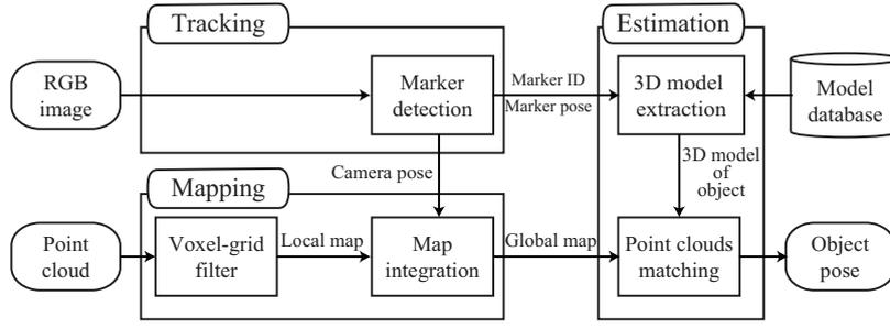
Fig. 1. Overview of our proposed method. Camera pose is tracked based on markers placed on objects in the *Tracking* part, and a global map is built by the integration of point clouds in the *Mapping* part. Finally, in *Estimation* part, the object's pose is estimated by the alignment of the global map and the object's shape model that has been preregistered in a database.
