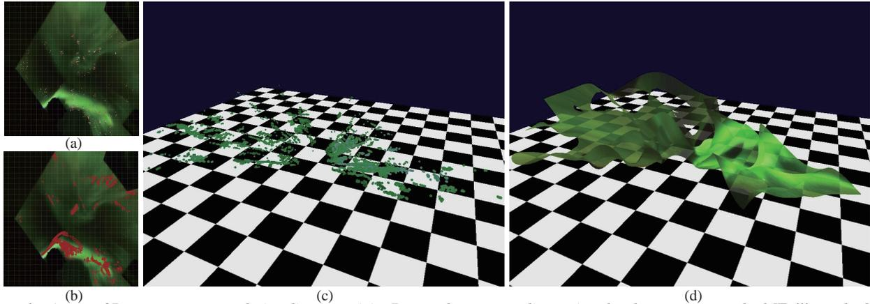
**Figure 1:** Aurora 3D measurement and visualization. (a): Detected corresponding points by the previous method [Fujii *et al.* 2014]. (b): Detected corresponding points by the proposed method after eliminating unreliable points by tracking feature points. (c): Aurora 3D visualization result by putting the detected points on 3D space. (d): Aurora 3D visualization result by using NURBS surface.
