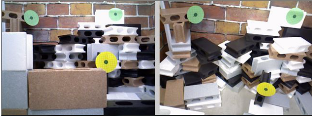
Fig. 3: Input images from the front sensor (left) and the arm sensor (right) at a certain moment. In the image from the front sensor, the background behind the obstacle can not be seen.
