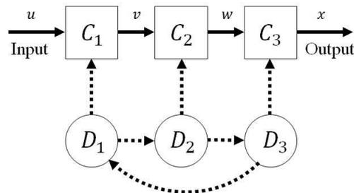
Fig. 1 This figure indicates an example architecture of electrical components and diagnosers in a robot system.  $C_n$  indicates a component, and  $D_n$  is a diagnoser. Arrow indicates correspondence relationship of fault diagnosis.
