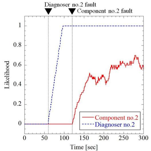
Fig. 3 Comparison of change of fault likelihood of diagnoser no.2 and component no.2.
