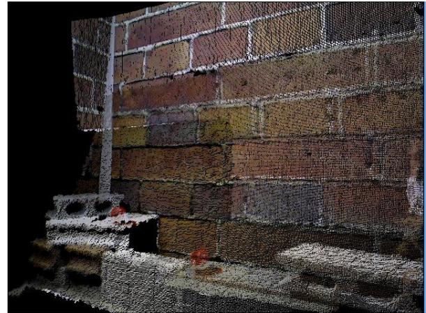
(a) An output image after moving the position of the virtual sensor without interpolation which was mentioned in Section III-C. The virtual sensor moved 0.15 m in the X direction and -0.15 m in the Y direction from the position of the front sensor, and rotated 30 deg about Z axis. In this picture, information of about 40 % of the field of view is missing.
