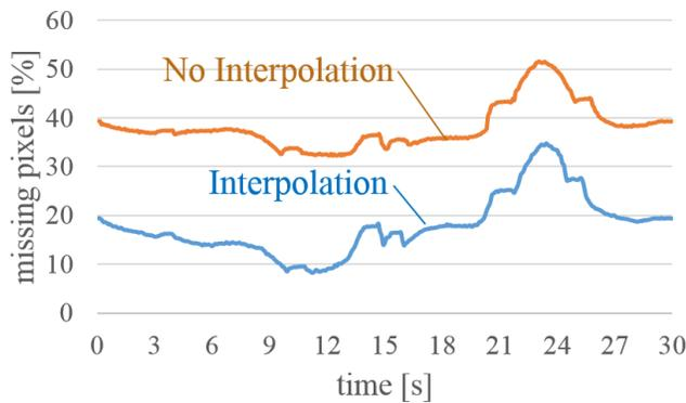
Fig. 8: The percentage of the missing pixels during the experiments. The evaluation was performed when the virtual sensor was located at the position in Fig. 7. The percentage improved after the simple interpolation explained in Section III-C.
