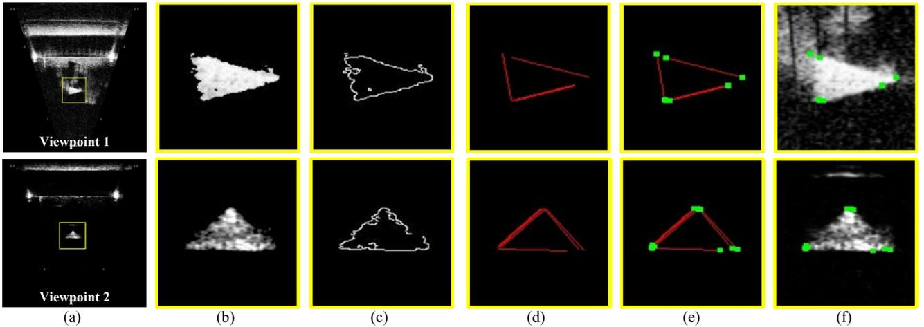
Figure 9. Feature extraction procedure and results from the triangular prism with respect to viewpoint 1 (top) and viewpoint 2 (bottom). Yellow squares represent the ROI: (a) original images, (b) designation of ROIs, (c) contours of the images extracted by Canny edge detection, (d) extraction of lines with a high level of confidence by probabilistic Hough transform, (e) extraction of endpoints of the lines as feature points, and (f) feature points on the original images.
