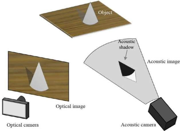
Figure 2. While optical cameras provide the same scenes as human sight, acoustic cameras provide significantly dissimilar images.
