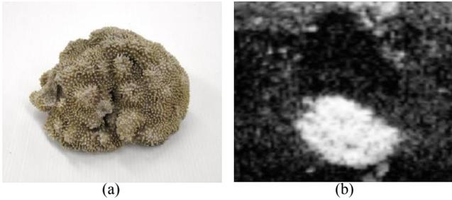
Figure 12. An example of difficult case to extract feature points from acoustic images: (a) an optical image of a coral and (b) a corresponding acoustic image.
