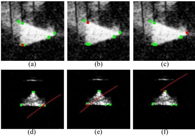
Figure 10. Finding correspondences between feature points: (a), (b), and (c) real acoustic images of the triangular prism with respect to viewpoint 1 and (d), (e), and (f) real acoustic images of the triangular prism with respect to viewpoint 2. The red point in (a) is a reference feature point to find the corresponding point in (d), and the red point in (d) is determined as corresponding by the red plotted line. Other correspondences can also be seen in (b), (e) and (c), (f).
