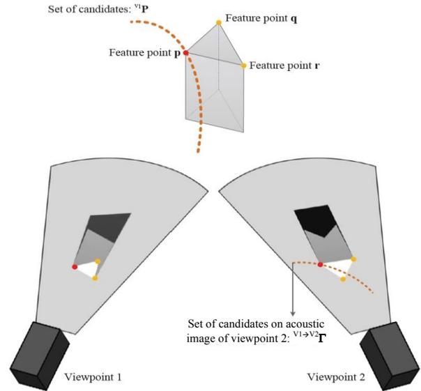
Figure 7. Conceptual image of the geometric design to find correspondences between feature points on each acoustic image.
