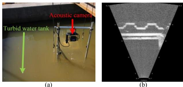
Figure 1. Because acoustic cameras provide acoustic images with accurate details, even in turbid water, they not only help with understanding the underwater situation but can also be applied to 3D measurement systems: (a) an acoustic camera system with ARIS in a turbid water tank and (b) an acoustic image of the turbid water tank bed.
