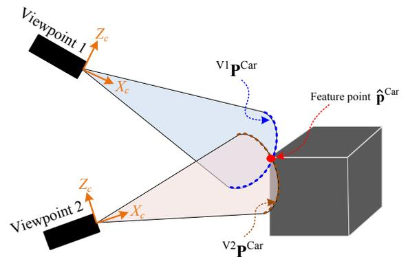
Figure 5. Conceptual image of the 3D measurement model using two acoustic viewpoints.
