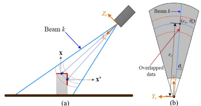
Figure 4. Overlapping phenomenon: (a) cross-sectional diagram of beam  $k$  and (b) pixels where acoustic pressure data overlap (red solid line). Because multiple acoustic pressure values overlap on the acoustic image when the detected points are located at the same distance from the acoustic camera in identical beam slices, the acoustic pressure values regarding the measurement points  $\mathbf{x}$  and  $\mathbf{x}'$  are output on the same pixel  $(r_c, \theta_c)$ .
