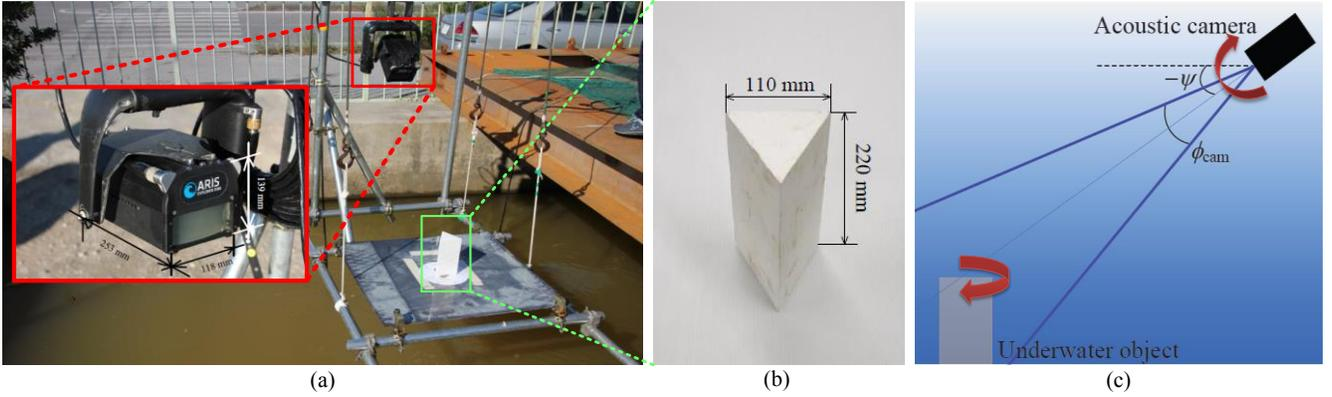
Figure 8. Experimental setup: (a) acoustic camera ARIS EXPLORER 3000 fixed to steel bar, (b) triangular prism used in the experiment, and (c) a conceptual image of environment settings for the experiment.
