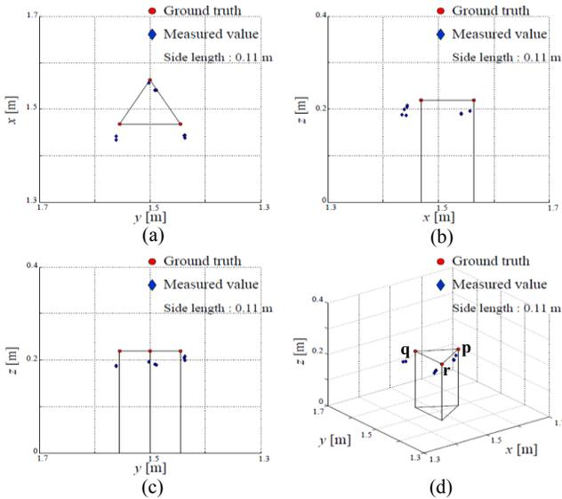
Figure 11. Experimental results for 3D measurement of the triangular prism. The 3D coordinates of the triangular prism's three vertices were measured from the real experiment: (a) 2D floorplan drawn on the  $x$ - $y$  plane, (b) 2-D floorplan drawn on the  $x$ - $z$  plane, (c) 2D floorplan drawn on the  $y$ - $z$  plane, and (d) projection plan. The red circles indicate the ground truth, and the blue diamonds indicate the measured values.
