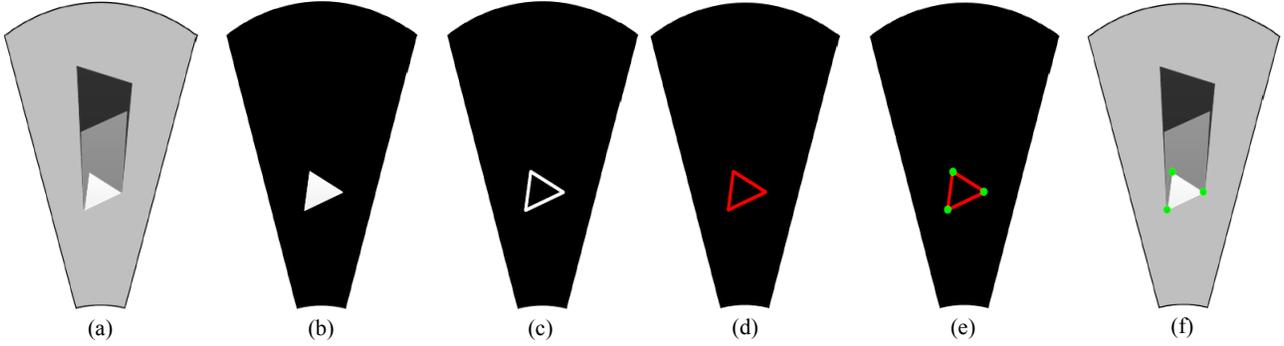
Figure 6. Process to extract feature points from an acoustic image: (a) original image, (b) designation of ROI, (c) contours of the image extracted by Canny edge detection, (d) extraction of lines with a high level of confidence by the probabilistic Hough transform, (e) extraction of endpoints of the lines as feature points, and (f) the feature points on the original image.
