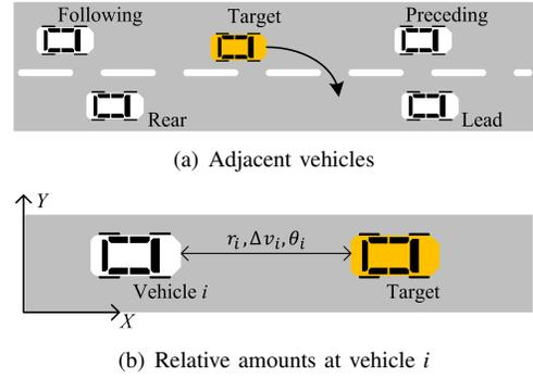
Fig. 4. Definition of adjacent vehicles and relative amounts
