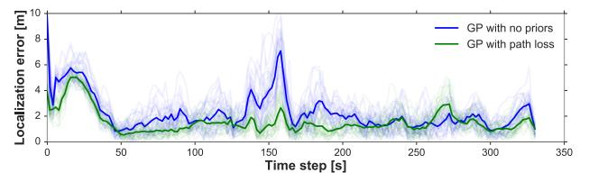
Fig. 5. Localization accuracy of our approach and a GP with zero mean when used as the perceptual likelihood of a dual MCL algorithm.
