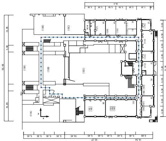
Fig. 3. Blue prints of the environment used for testing. The blue line and blue dots show the route taken by the robot when mapping and localizing, and purple dots indicate the *anchor* points used for rectifying odometry.
