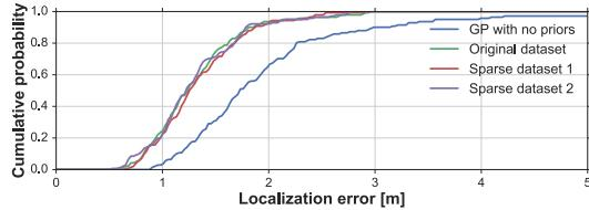
Fig. 7. Cumulative probability of localization accuracy for training datasets with 1.658, 3.276 and 4.849 m.
