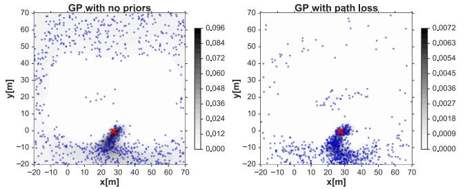
Fig. 4. Posterior probability distributions for (left) a GP with no priors and (right) our approach. Red X represents true location, shaded areas represent posterior probability values (lighter ones represent low probability, while darker ones, high), blue dots represent samples taken from the distribution.
