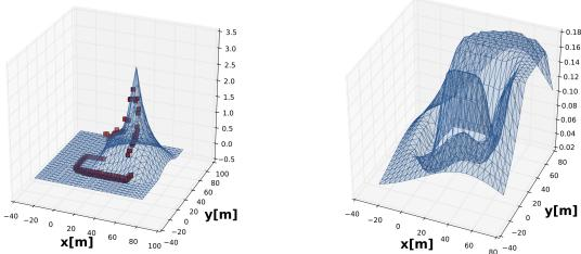
Fig. 2. Propagation model used for likelihood calculation of new RSS measurements. Figure shows (left) the predicted mean and (right) the predicted variance for the access point.
