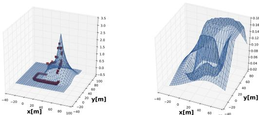
Fig. 2. Propagation model used for likelihood calculation of new RSS measurements. Figure shows (left) the predicted mean and (right) the predicted variance for the access point.
