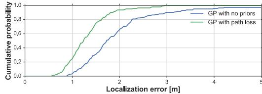
Fig. 6. Cumulative probability of localization accuracy once the dual MCL has converged, comparing our approach and a GP without priors.
