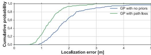
Fig. 6. Cumulative probability of localization accuracy once the dual MCL has converged, comparing our approach and a GP without priors.
