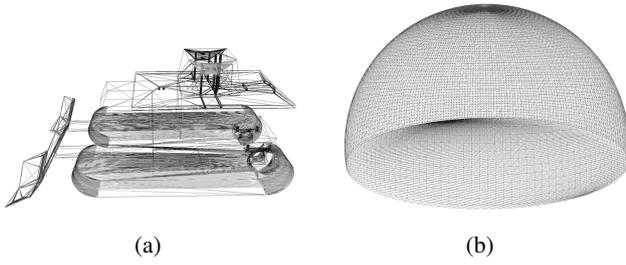
Fig. 1: (a) The mesh model of the construction machine is built by CAD data. Thus the mesh model of the construction machine can be built in proper precision. (b) The surrounding environment is approximated as a semi-sphere mesh model, because the surrounding environment of construction work sites is usually spacious and unable to be measured.
