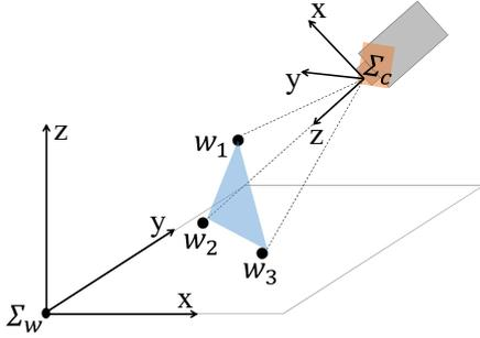
Fig. 4: The world coordinate system is denoted as  $\Sigma_w$ . The local fish-eye camera coordinate system is denoted as  $\Sigma_c$ . The extrinsic parameters between the local fish-eye camera coordinate system and the world coordinate system can be estimated by using three known points  $w_1, w_2, w_3$ .
