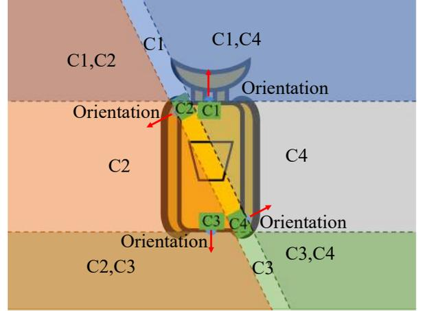
Fig. 7: Positions and orientations of  $C_i$  ( $i = 1, 2, 3, 4$ ). Four mounted fish-eye cameras numbered in the order of counterclockwise. The color shadows: blue, orange, green, and gray show the visible region of each fish-eye camera. The common visible region of every two fish-eye cameras labeled in  $C_i, C_j$  ( $i, j = 1, 2, 3, 4$ ). The orientations of the fish-eye cameras are shown as the red arrows.
