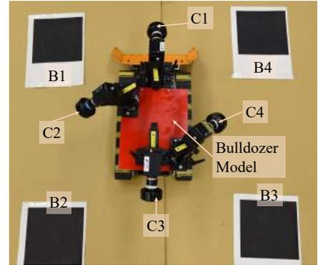
Fig. 8: Installation angle of fish-eye cameras. The left side and right side installation angle of fish-eye camera were adjusted to 45° lower than horizontal direction. The front side and back side installation angle of fish-eye camera adjusted to 10° lower than horizontal direction. Four square boards  $B_i$  ( $i = 1, 2, 3, 4$ ) were placed in common visible region of every two fish-eye cameras in a counter-clockwise order.
