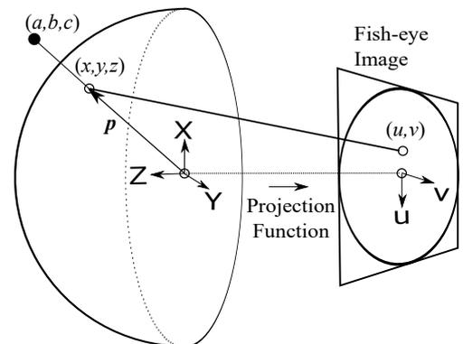
Fig. 3: A three-dimensional point  $(a,b,c)$  in the world coordinate system is projected as a direction vector  $\mathbf{p}$  in local fish-eye coordinate system on the spherical camera model. Also, it is projected to coordinate  $(u,v)$  in the fish-eye image.
