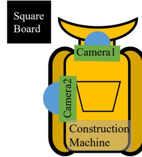
Fig. 5: Square boards are used for estimating the extrinsic parameters between the local fish-eye camera coordinate system and the surrounding environment mesh model coordinate system. In order to estimate the extrinsic parameters between the local fish-eye camera coordinate systems of camera 1 and camera 2, a square board is placed in the common visible region of camera 1 and camera 2.
