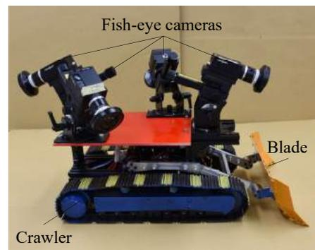
Fig. 6: Experiment was performed with this bulldozer model. The color of the bulldozer model was changed in order to be exhibited clearly. The upper part of the bulldozer was painted in red, the blade part was painted in orange, and the crawler parts were painted in blue and yellow. This bulldozer model is powered by AC adapters of 5 V and 12 V, and controlled by a USB gamepad.
