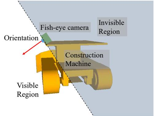
Fig. 2: In order to obtain the actual scene images of both the construction machine and the surrounding environment, fish-eye cameras are adjusted to downward directions. The visible region of left side mounted fish-eye camera is the non-shadow part after the installation angle of fish-eye camera is adjusted to a lower diagonal direction. The red arrow shows the the orientation of the fish-eye camera.
