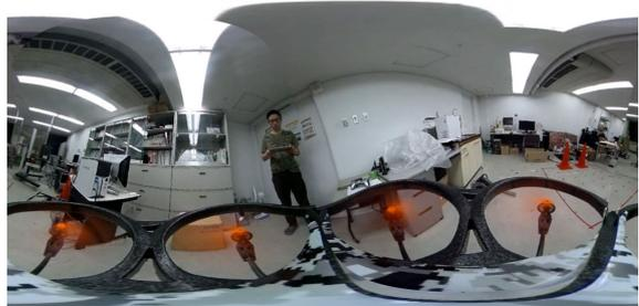
(b) An original equirectangular image from the mounted Ricoh Theta. Here, the drone body severely occludes the camera vision.
