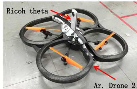
(a) An example of mounting a spherical camera, Ricoh Theta, on the body of an AR.Drone 2.
