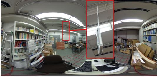
Fig. 8. Experimental setting to record ground truth image frames. A spherical camera, Ricoh Theta, is hung using a thin string to take ground truth image sequences.
