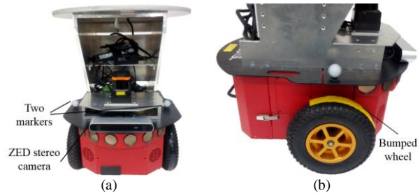
Fig. 1: Pioneer 3-DX robot. a) The ZED stereo camera and the motion capture's markers. b) System fault: a bumped wheel.
